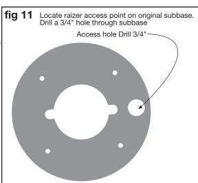
NOTE: This router requires a 3/4" pocket or use of 8" X 8" black rubber spacer for router table installation. Pages 4,5,6.
